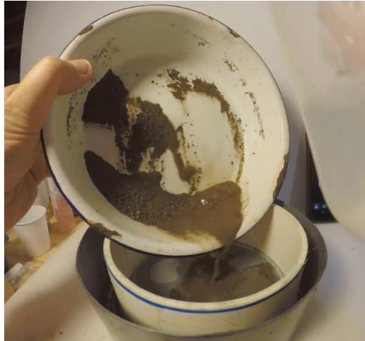
Figure 14. Rinsing all the material <2mm into the 250 micron sieve to perform the next wash of stable aggregates at the 250 micron size.
