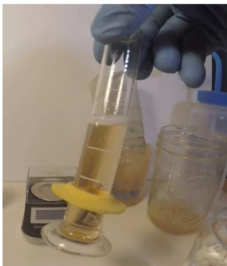
Figure 35. The extracted, filtered solution has been acidified and brought to a standard volume of 20 mL. It is ready for reacting with the color reagent to develop the blue color and then read with the colorimeter.
