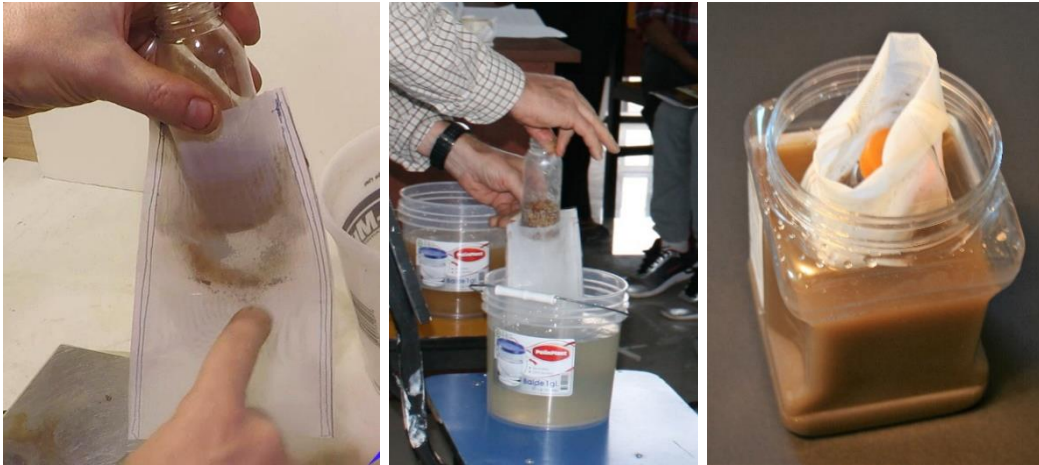
Figure 19. Washing the soil in the bottle and bag combination. After a minute or so, clays and silt will have moved outside that bag and the water will become quite cloudy (right-hand image)
