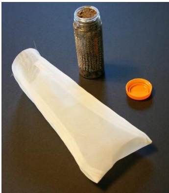
Figure 17. The mesh bag from 250-micron mesh and a bottle big enough for sieving 100g of soil, with 2mm holes drilled into the side of the bottle with a drill or hot nail.
