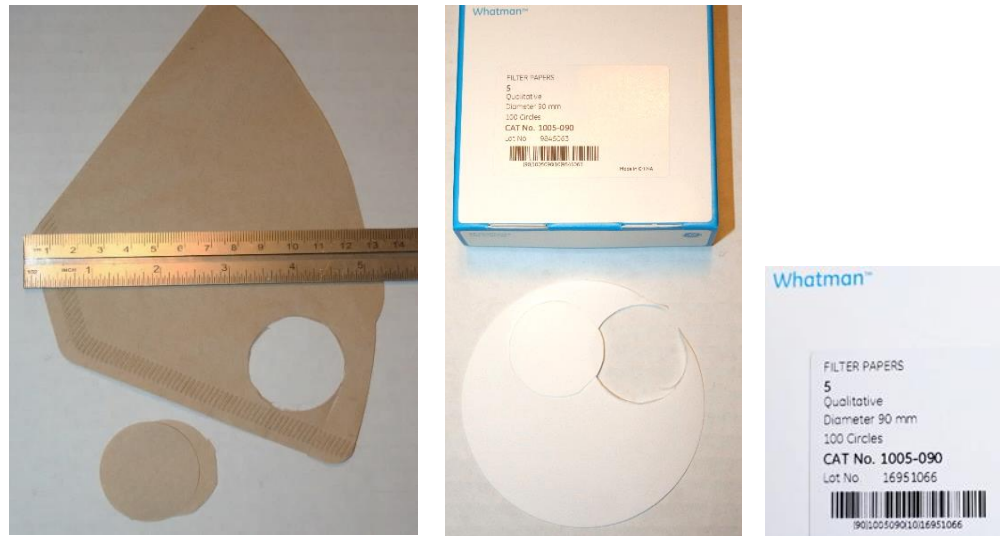
Fig. 4. Left: cone coffee filters; Right: lab-quality filters, Whatman type #5 with 2.5 \mu\text{m} pores. Circles with diameter \sim 3\text{cm} are cut to use in a filtering rig, or the entire filter folded into a funnel.
