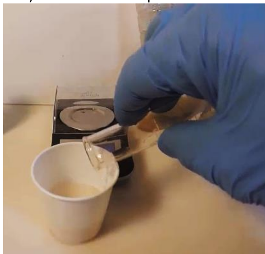
Figure 34. Mixing 3 mL solution of sodium bisulfate (15g NaHSO 4 per 100 mL) to acidify 7 mL of filtered extract. Note the bubbling of the soil extract as bicarbonate reacts with the acidic bisulfate.
