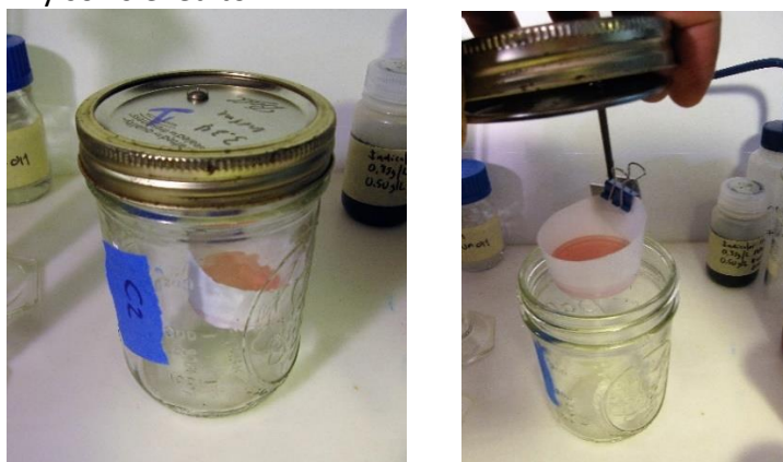
Figure 38. Design of a 500 mL jar with a small plastic cup suspended inside containing the boric acid trap solution. Soil being digested by 2M sodium hydroxide solution at 48°C is placed on the bottom of the jar below the cup.
