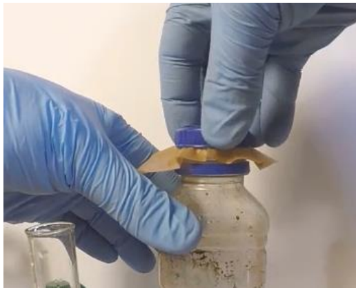
Figure 31. Placing a double layer of coffee filter paper below the lid of the bottle.
