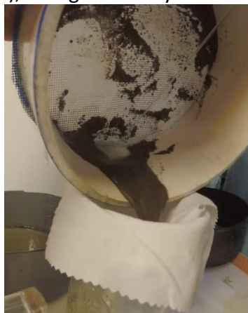
Figure 15. Washing a stable aggregate fraction from the sieve to a funnel with a cloth to retain the soil for drying and weighing.
