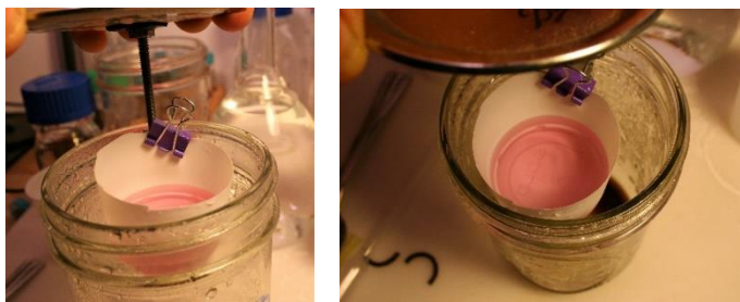
Figure 37. view of the test jar before closing the jar and incubation, note dark soil + NaOH solution at bottom of jar and small cup of boric acid color indicator suspended above.
