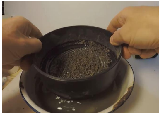
Figure 13. Left, Lowering and raising the sieve 50 times in two minutes. At right, a metronome app for cell phone to regulate the pace of dipping the sieve into the water.
