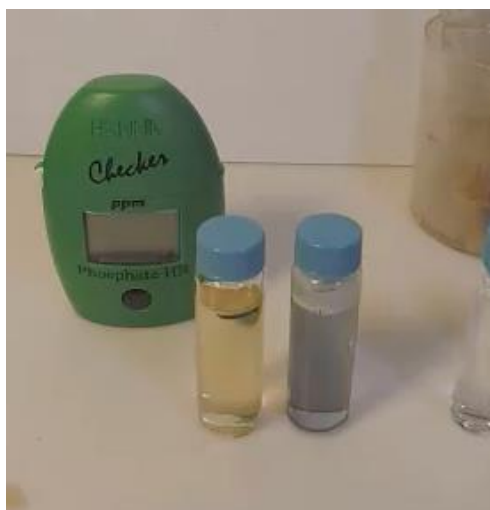
Figure 37. A blue color will develop in the extract with the reagent packet added. The other yellow colored vial serves as the color blank to be measured in the colorimeter.
