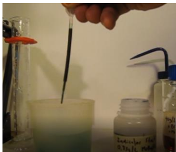
Figure 40. Adding 4 mL indicated stock solution to 196 mL water to create the final concentration of pH indicator, before adding boric acid.
