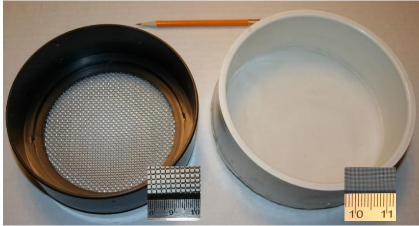
Figure 5. Left: low-cost plastic sieve with 2mm hole size; Right: Home-made 250-micron sieve using #60 mesh from the silk-screening industry, made with a large-diameter plastic tube as a frame. Rulers shown on enlarged insets use cm units, with small millimeter ticks.
