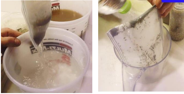
Figure 21. Washing the mesh bag a last time in clean water (left) before washing the material inside the bag to a beaker or other cup with a spout for decanting (right).
