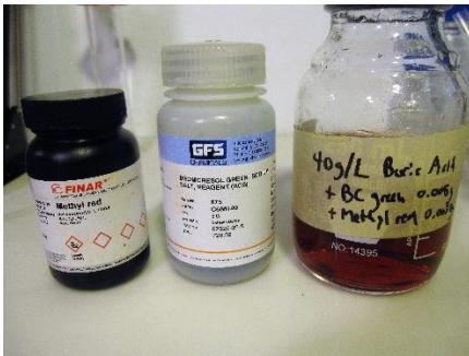
Figure 39. The color indicators Methyl Red and Bromocresol Green. Very tiny amounts of each are needed to make the indicator solutions.
