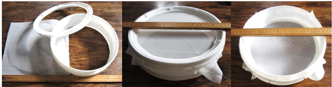
Figure 6. Creation of a 250 micron sieve from the top section and lid of a 5-liter paint bucket with a heavy snap-on lid. Mesh used for screen printing with a hole size of 250 microns is sandwiched between the top rim of the bucket and the snap-on lid. When the lid is snapped on, the mesh is tensioned to provide a very effective sieving surface.
