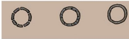
Figure 8. The FAO feel test for soil texture: a sequence of tests performed on a kneaded ball of moistened soil, which can be used to classify soil textural type in the FAO “feel method”
