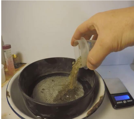
Figure 12. Adding coarse sieved soil (sieved to ~10 mm) to the 2mm sieve in a basin of water.
