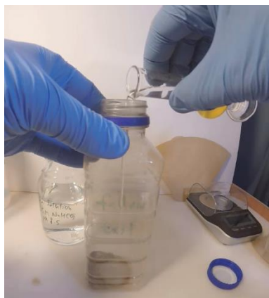
Figure 29. Adding 25 mL Olsen solution to the soil in a re-used juice bottle to start the extraction.
