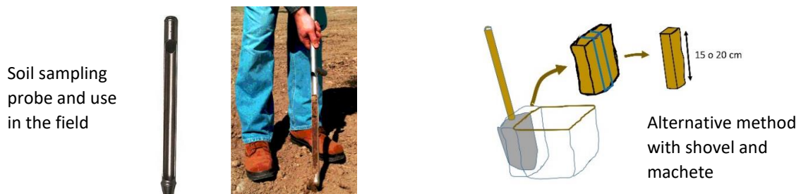
Figure 1.1. Two methods to sample soil: Left: a soil sampling tube or probe; Right: using a shovel to cut a slice and then trim it into a square column with an even mix of depths.
