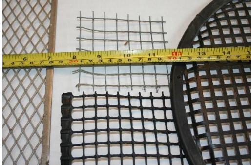
Fig. 10. Examples of different types of mesh that can be used for pre-screening dry soil, with a hole size between 8 and 12 mm.
