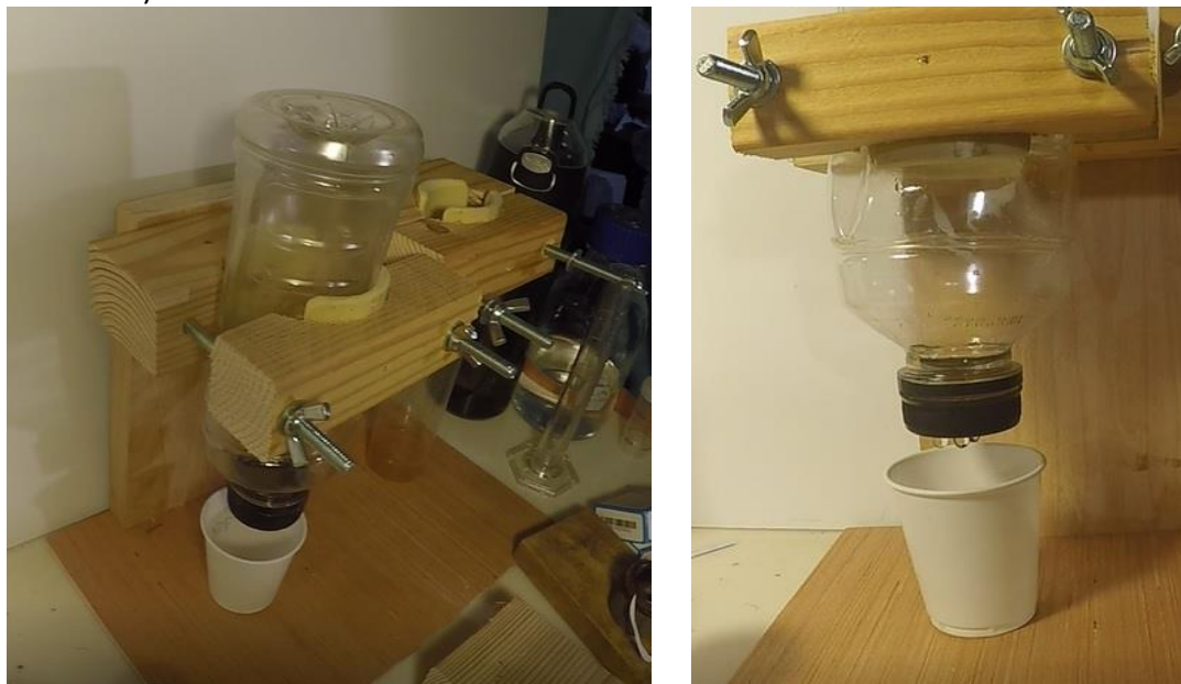
Figure 33. A bottle press to help with filtration using bottles and filter paper in the lids, which allows maintaining pressure on the bottles and use a laboratory filter or a coffee filter to extract the clays from the extract. This approach saves time because while pressing the bottles one can proceed with other tasks.
