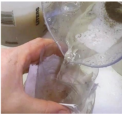
Figure 22. Decanting the floating POM into a cloth that is mounted on a plastic cylinder made by cutting a plastic jar or bottle.
